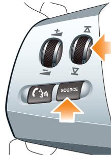
2. To make or receive a call, press
