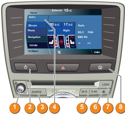
1. Press to switch audio on/off. Rotate for volume.
