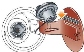
A hook is provided on the flap hinge to hold the cap whilst refuelling. After refuelling, tighten the cap until it clicks three times.
