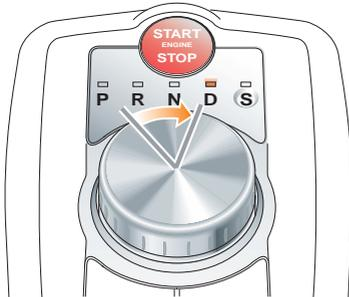
The ignition must be on and the footbrake depressed before the selector can be rotated from the **Park** position. Maintain brake pressure until a gear is selected.
