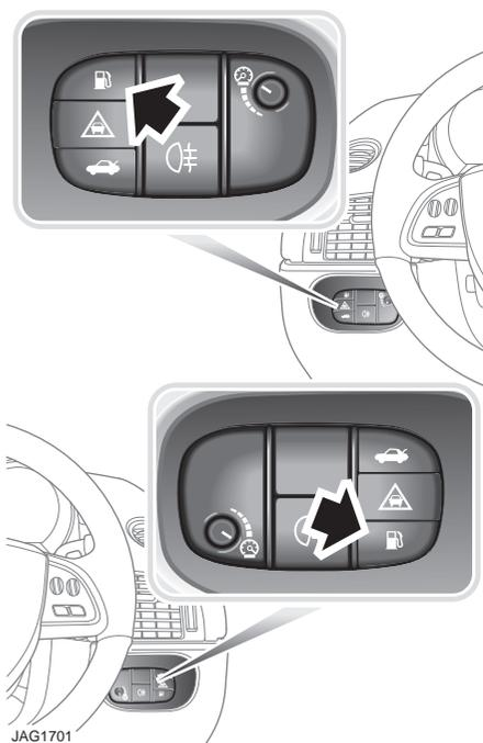
The filler flap release switch is located in the switchpack below the facia. The switch is inhibited if the vehicle is armed. The filler flap is on the right-hand side of the vehicle.
