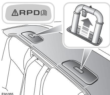
If the sensors determine that a risk of rollover is imminent, the RPD will be deployed.
