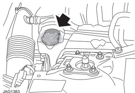
1. With the ignition on, but the engine not running, unscrew the oil filler cap (arrowed).
