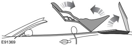
4. The rear quarter windows open, an audible warning sounds and the top unlatches and starts to move. The tonneau closing panel opens (the front windows will fully open. The door window switch will require to be pressed to close the windows).
