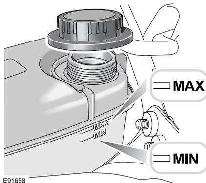
Ensure the coolant level is maintained between the **MAX** and **MIN** level indicators, located on the side of the expansion tank.
