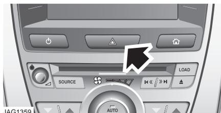
If the vehicle is stationary in an unsafe location, or may cause a hazard to other road users, switch on the hazard warning flashers. Press the switch to turn the hazard warning lamps on.
