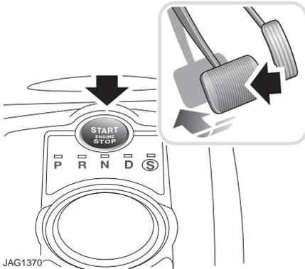
With the brake pedal applied, press and release the START/STOP button. The engine will start and all systems will become functional.
