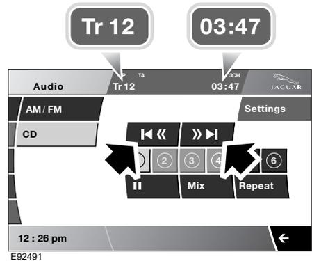
**Seek down and seek up buttons (arrowed):**
