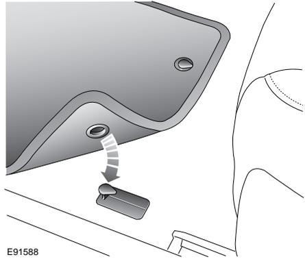
The driver's floor mat must be correctly positioned and secured under the tongues on the retention posts (only one post shown). Ensure that the mat does not interfere with the operation of the accelerator or brake pedal.
