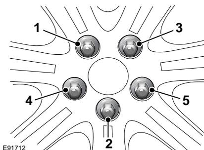
Using the wheel nut wrench, lightly tighten the wheel nuts alternately using the sequence shown in the illustration.
