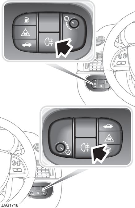
The rear fog lamps can only be switched on if the low beam headlamps are on.
