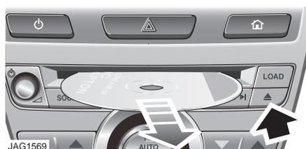
Press the eject button. A short press will eject a single CD, a long press will eject each loaded CD in turn (six disc players only).
