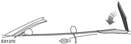
5. When the top is fully open, the audible warning sounds again. The tonneau closing panel is fully automated and encloses the convertible top in the stowed position.
