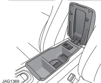
The sliding armrest is hinged at the rear and has a release button located on the front of the armrest.
