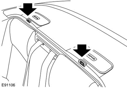
Two child restraint anchorages are provided. These are located under top tether covers in the rear tonneau.
