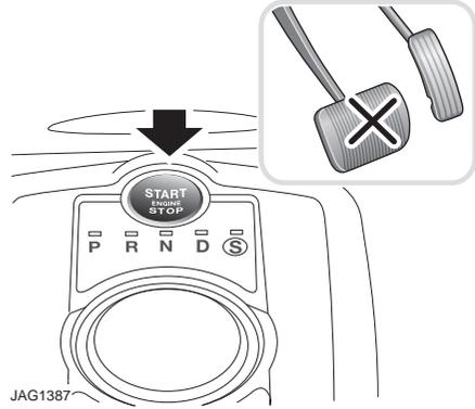
To turn on the ignition system without starting the engine, press the START/STOP button without pressing the brake pedal. All systems will become functional.
