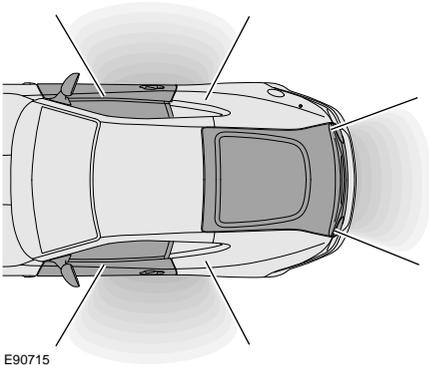
Keyless entry allows the driver to unlock and disarm the vehicle by simply operating the door handle. The keyless entry function operates as follows:
