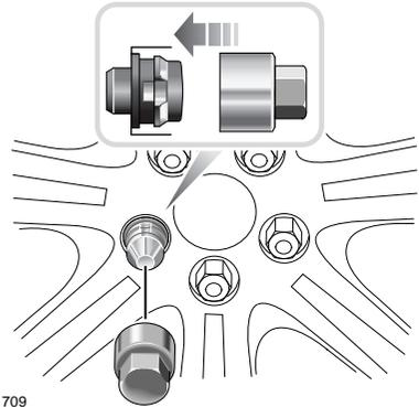
1. Insert the adaptor firmly onto the locking wheel nut.
