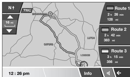
The three routes are shown in three different colours. Three corresponding boxes showing the route details, are also displayed.
