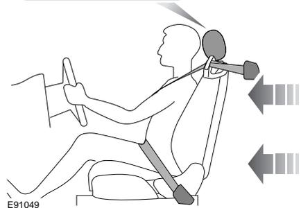
Both front seats are equipped with Active Head Restraints (AHR) which reduce the risk of neck and spinal injury (whiplash) in the event of a rear impact. When activated, the head restraint moves upwards and forwards, supporting the occupant's head.
