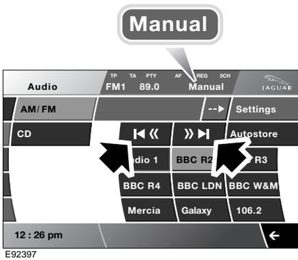
**Long press:** In AM or FM mode, for as long as the button is being touched, the frequencies will be scanned either up or down.
