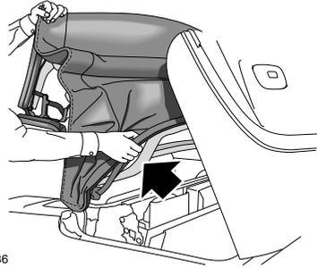
7. Ensure that the tension bow is fully raised.
