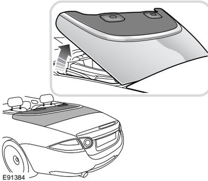
5. Fully open the tonneau panel. It will self-support when fully opened.
