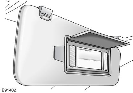
Adjustable sun visors can be swung downwards or unclipped and swung sideways to reduce sun glare.
