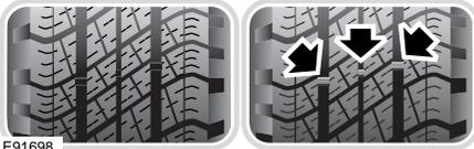
When the tread has worn down to approximately 2mm, wear indicators start to appear at the surface of the tread pattern. This produces a continuous band of rubber across the tread, as a visual indicator.
