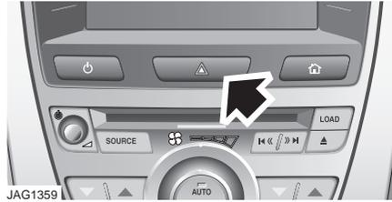
Press the switch to turn the hazard warning lamps on. When the hazard warning flashers are operating, the indicator warning lamps will flash in time with the hazard warning flashers.
