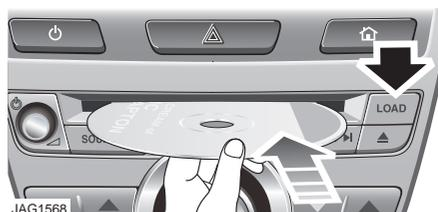
Press the **LOAD** button and insert each CD into the CD slot, as requested by the displayed message. A pop-up message on the screen will indicate which slot is being selected, until the unit is fully loaded.
