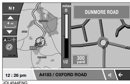
As you approach a junction, in addition to the voice guidance, an inset on the map will display an enlarged view of the junction.
