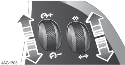
Briefly rotate the speed adjust control upwards (+), to store the speed in the memory and engage the system.
