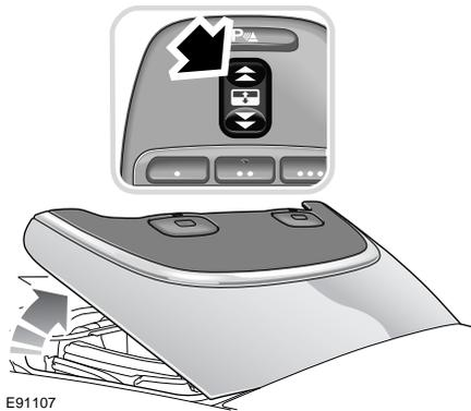
1. Open the tonneau panel by briefly pressing and holding the front of the convertible top overhead console switch.
