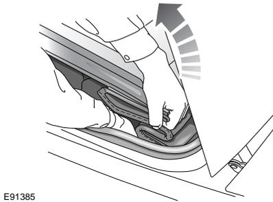
6. From the left-hand side of the vehicle, place your right hand down the side of the folded convertible top. Ensure that the bottom of the convertible top, which includes the tension bow, is securely held. Securely hold the convertible top header assembly with your left hand. With both hands pull the whole of the convertible top up and forward.
