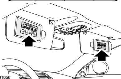
Airbag warning information is printed on the driver's and passenger's sun visor.
