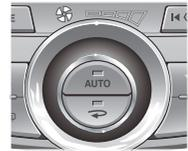
Set the blower speed by adjusting the AUTO rotary control knob.
