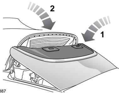
8. Supporting the tension bow, lower the tonneau panel (1). Then lower the tension bow (2) onto the tonneau panel.
