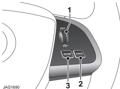
The cruise (speed) control system can be used by the driver to maintain a selected vehicle speed without the driver having to use the accelerator.
