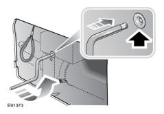
**3.** Insert the Allen key into the pump and rotate anticlockwise (approximately one turn).
