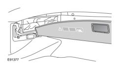
A luggage separator is located in the luggage compartment, to prevent items from moving into the area where the convertible top is stowed.
