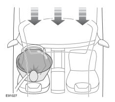
With a front impact of sufficient force. the restraints system will trigger the front airbag(s) and seat belt pretensioners, which immediately tighten the seat belts.
