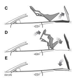
Lift the tonneau cover fully and support (**C**). Pull the convertible top rearwards and downwards (**D**) so that it is fully stowed.
