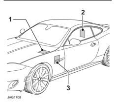
There are three separate fuse boxes fitted to the vehicle, each one containing fuses protecting a different group of circuits.
