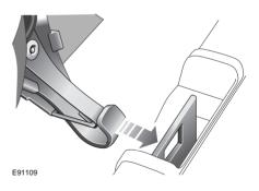
**4.** Attach the child restraint top tether clip to the top tether anchorage bracket.
