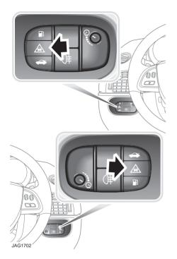
This Forward Alert feature may be switched on or off using the Forward Alert switch in the lower outboard knee bolster switchpack.
