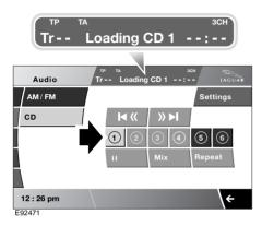
When a CD has been selected (arrowed), the upper display indicates which disc is being loaded and will commence playing when loading has been completed.
