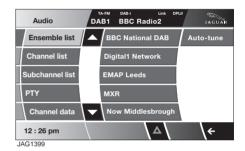
Select **Ensemble list** to display a list of all available ensembles. Select an ensemble name in the list to display a list of channels in that ensemble. Select a channel name to tune that channel.
