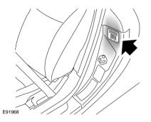
Vehicles have the Certification Label adhered to the left-hand rear door post (right-hand rear door post China only). Vehicle weights, paint code, manufacture date and the Vehicle Identification Number (VIN) are shown on this plate.
