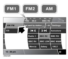
Touching and releasing the **AM/FM** button, will cycle the radio through FM1, FM2 and AM (a combination of Medium and Long wavebands). Band selection will be shown in the display panel. When a CD is being played, pressing the band switch will select radio operation.
