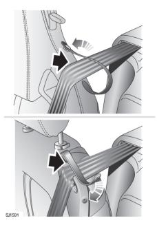
To assist with both access and positioning of the front seat belt webbing, a guide-retainer is incorporated into each front seat.
