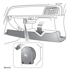
An electrical accessory socket is located inside the glove compartment. This 12 volt socket should only be used for the temporary connection of electrical items, such as a vacuum cleaner or cool box.
