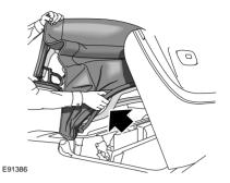
7. Ensure that the tension bow is fully raised.
