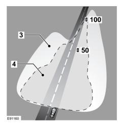
Xenon lamps (**3**) provide significantly improved visibility over halogen lamps (**4**).
