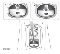
The switch which operates the parking brake is mounted on the centre console to the rear of the gear selector.
