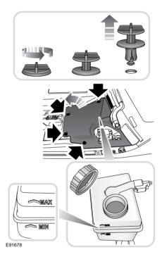
Remove the four fixings securing the cover panel.
