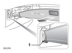
Pull the handle on the luggage separator towards you. There is a lug on either side of the luggage separator: slide the lugs into the sliders on either side of the luggage compartment. The luggage separator will positively locate in the vertical position. A proximity switch (1) is located in the separator assembly, so that the convertible top will not open and retract until the separator is in the fully deployed position.
