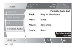
Touch and hold (two seconds) the --> button to display the **Portable audio text** pop-up screen providing all the id3 tag information available for the track.
