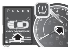
If the telltale light illuminates, you should stop and check your tyres as soon as possible and inflate them to the recommended pressure as stated on the tyre pressure placard fixed to the end of the left-hand side door. If low pressure warnings occur frequently, the cause must be determined and rectified.
