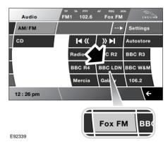
After tuning to a station, touch and hold (2 seconds) the selected button until the station has been stored. A station can be recalled from the preset memory by touching and releasing the button.
