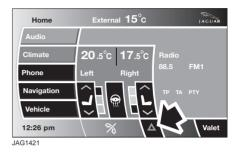
When a message is displayed in the message centre (e.g. WASHER FLUID LOW), a red warning triangle icon appears on the touch-screen, where shown.
