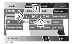
If subchannels are available under the current channel, the subchannel arrow icon (1) is displayed at the top of the touch-screen and the Subchannel button is enabled.
