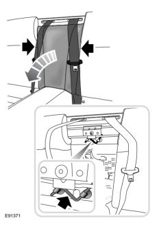
Remove the Allen key from its stowed position, behind the rear seat centre section, by grasping the sides of the section, as shown, and pulling sharply.
