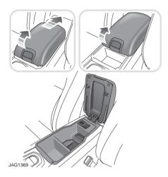
The sliding armrest is hinged at the rear and has a release button located on the front of the armrest.
