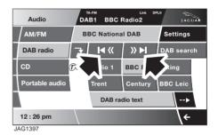
Briefly touch one of the channel seek buttons to select the next available digital channel. The seek up button selects the next channel, the seek down button selects the previous channel.
