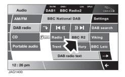
Store up to eighteen digital channels (six each on **DAB1**, **DAB2** and **DAB3**) using the numbered preset keys. Follow the procedure below to store channels as presets.
