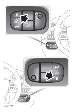
The filler flap release switch is located in the switchpack below the facia. The switch is inhibited if the vehicle is armed. The filler flap is on the right-hand side of the vehicle.
