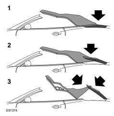
The convertible top and tonneau cover movement can cease in any of the positions 1, 2 or 3, as shown.
