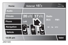
With the engine running, touch the steering wheel icon to turn the steering wheel heater on or off.
