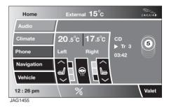
The Home menu will indicate whether a CD is loaded and, where applicable, which CD slot is loaded and ready for playing. If no CDs have been loaded, the touch-screen displays ghosted discs.
