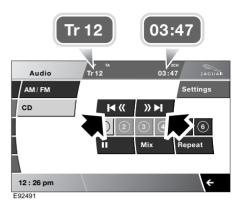
Seek down and seek up buttons (arrowed):
