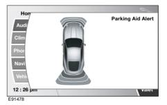
When the reverse parking aid is active, a pop-up screen is initiated displaying the area of the vehicle. This can be cancelled by touching the screen within the pop-up area.
