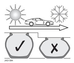
In order to minimise this effect, tyre pressures can be adjusted to compensate before the start of the journey. Alternatively, tyre pressures can be adjusted when the area of lower ambient temperature is reached.
