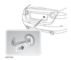
The luggage compartment emergency key barrel is located behind the rear license plate.
