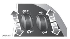
Briefly rotate the speed adjust control upwards (+), to store the speed in the memory and engage the system.
