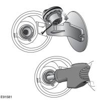
To remove the filler cap, turn it anticlockwise approximately a ¼ turn, until a slight resistance is met. Continue turning to release it. Remove the cap from the filler neck.
