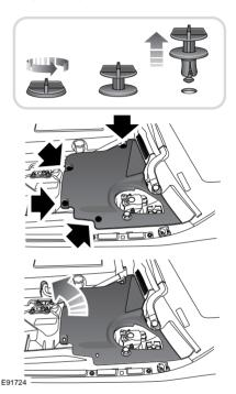
Remove the engine compartment left-hand cover.
