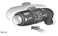
**High beam:** With the headlamps on, push the switch away from the steering wheel to switch to high beam.
