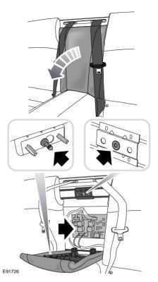
A fuse box is located behind the rear seat centre section.
