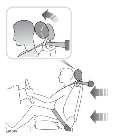
Both front seats are equipped with Active Head Restraints (AHR) which reduce the risk of neck and spinal injury (whiplash) in the event of a rear impact. When activated, the head restraint moves upwards and forwards, supporting the occupant's head.
