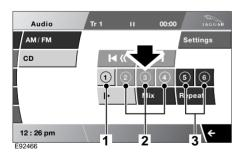
From the CD player touch-screen, select an empty slot (2). A message indicates to insert the CD into the loading slot. Load the CD.
