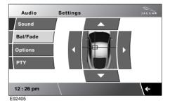
**Bal/Fade:** From the audio menu, select **Bal/Fade**. Touch the arrow buttons to optimise the Balance (left to right) and Fade (front to rear) settings.
