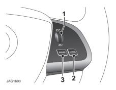
The cruise (speed) control system can be used by the driver to maintain a selected vehicle speed without the driver having to use the accelerator.
