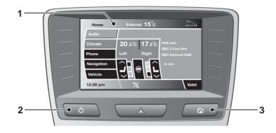
**Note:** When the engine is stopped, for the touch-screen to remain active, press the engine START/STOP button again without pressing the brake pedal (ignition system on).
