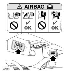
Airbag warning information is printed on the driver's and passenger's sun visor.
