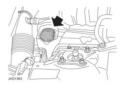
With the ignition on, but the engine not running, unscrew the oil filler cap (arrowed).
