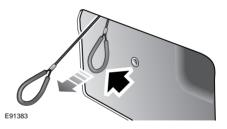
Pull the tonneau release cable, until fully 4. extended. Close the luggage compartment lid.
