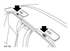
Two child restraint anchorages are provided. These are located under top tether covers in the rear tonneau.
