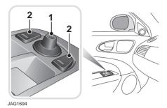
Both door mirrors are adjusted from the driver's door control panel.
