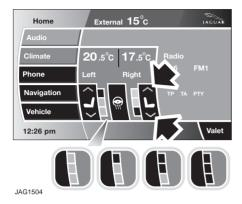
**Note:** To prevent the battery from becoming discharged, the climate seats will only operate when the engine is running.
