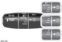
Three settings on the rotary collar set the time that the headlamps will remain on after the driver's door has closed:
