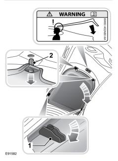
The luggage cover is removed by releasing the two latches (1) on either side of the luggage cover and sliding the cover downwards and forwards, so that the rear locating pegs (2) are disengaged from the trim and body. This will allow the luggage cover to be completely removed.
