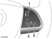
**1**. The speed adjustment control thumb wheel is used to engage cruise control initially, by rolling it upwards. It is also used to increase (+) or decrease (-) the set speed, until the desired speed is obtained.
