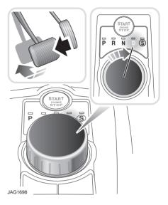
To select Drive (**D**) when the vehicle is stationary:-
