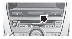
If the vehicle is stationary in an unsafe location. or may cause a hazard to other road users. switch on the hazard warning flashers. Press the switch to turn the hazard warning lamps on.
