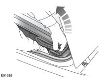
6. From the left-hand side of the vehicle, place your right hand down the side of the folded convertible top. Ensure that the bottom of the convertible top, which includes the tension bow, is securely held. Securely hold the convertible top header assembly with your left hand. With both hands pull the whole of the convertible top up and forward.
