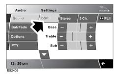
**DSP (Digital Signal Processing):** To optimise the sound for specific seating positions, select **DSP**.
