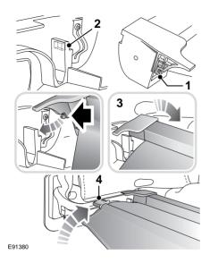
With the partition slightly extracted, position the luggage separator up to the support brackets, with the front edge raised. Ensuring that for both sides, the catch (1) will engage in the locating slot (2), rotate the main body of the luggage separator (3), so that it sits down into the support brackets. Fit the partition lugs into the sliders (4) and retract the luggage separator partition into the normal stowage position.
