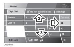
If you do not wish to be disturbed by incoming phone calls, select the bell icon (1) on the touch-screen. A visual representation will be displayed on the touch-screen, to advise the driver that the Do not disturb mode is selected (3) and **Do not disturb mode** will be visible when in telephone mode (2). Any incoming calls will be rejected or diverted to voice mail.
