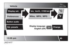
To change the units: The unit choices are selected by touching the relevant button (either km, km/h, I/100 km, or Miles. MPH, MPG).
