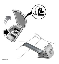
The top tether anchorages are positioned on the rear parcel shelf, under access covers, at the centre-line of each rear seating position.
