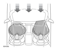
The passenger airbag is fitted and stowed above the glove compartment. This panel is marked AIBBAG, See OCCUPANT SENSING (page 44).
