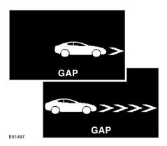
The message centre will display the gap set. The shortest (Gap 1), represented by 1 chevron, and the longest (Gap 4), represented by 4 chevrons, are illustrated above.
