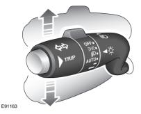
The direction indicators are operated using the indicator stalk. Move the stalk up or down, to indicate a right or left turn. A green warning indicator will flash in the instrument panel.
