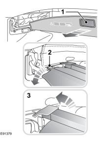
With the luggage separator in the stowed position, pull the handle towards you (1) and disengage the lugs from the sliders (2).
