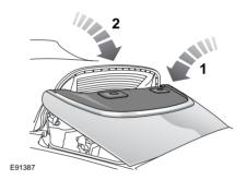
Supporting the tension bow, lower the tonneau panel (1). Then lower the tension bow (2) onto the tonneau panel.
