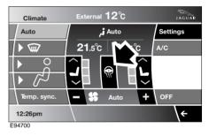
The heated steering wheel can also be activated in the same way via the Climate menu.
