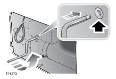
Insert the Allen key into the pump and rotate anticlockwise (approximately one turn).
