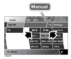
**Long press:** In AM or FM mode, for as long as the button is being touched, the frequencies will be scanned either up or down.
