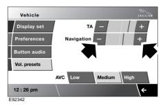
This level can be adjusted by setting the volume level on the **Vehicles - Syst. settings - Vol. presets** screen or, by turning the volume rotary control knob during the traffic announcement.
