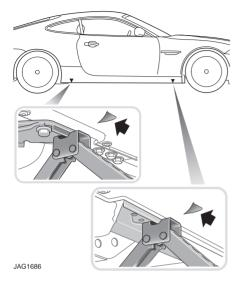
The simplest way to correctly locate the jacking point is to feel along the sill panel to the triangular indentation and then fit the jack to the body, not to the sill panel.
