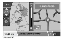
As you approach a junction, in addition to the voice guidance, an inset on the map will display an enlarged view of the junction.
