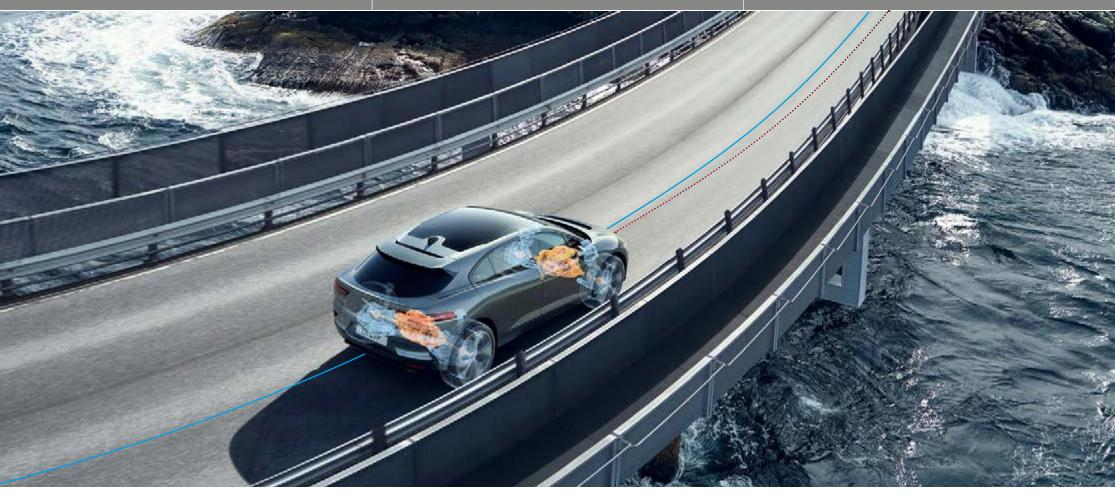
Torque Vectoring by Braking applies brake pressure to slow the inside front or inside rear wheels independently helping to prevent understeer and stay on the true line of travel.
