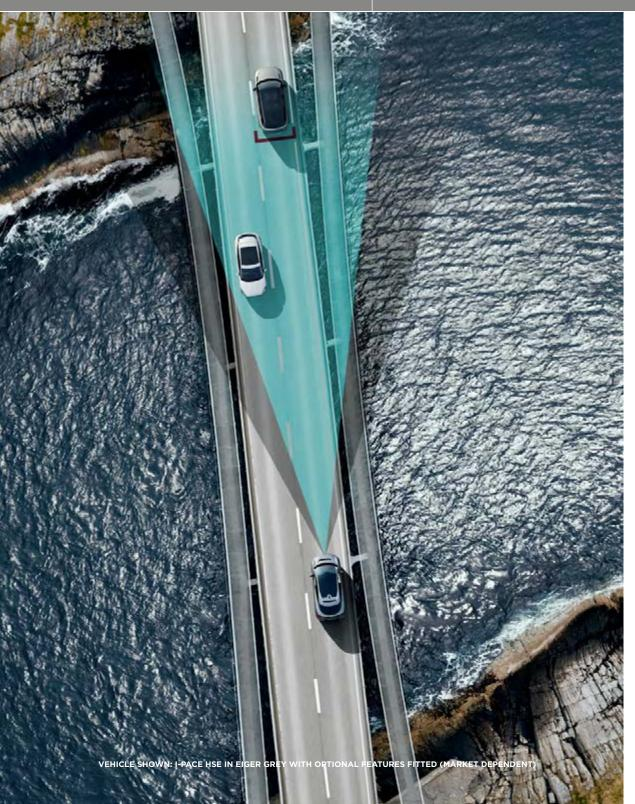
Adaptive Cruise Control keeps you at a safe distance from the vehicle in front even when it slows. Should it stop completely, you will come to a smooth halt behind it. In stop-start traffic, Adaptive Cruise Control will automatically resume following the car in front.
